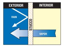
The Loxon system allows the coating to resist wind-driven rain when two coats are applied. It also allows the masorry structure to release moisture vapors without interfering with the adhesion and the performance of the coating.
